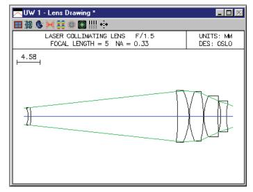
We will compute the sensitivity of the on-axis RMS OPD to decentration of the five components in the lens. We assign a trial decentration tolerance of 10  $\mu$ m to surfaces 2, 4, 6, 8, and 10 (i.e., the front surfaces of the components). OSLO assumes that the component decentrations have a Gaussian distribution that is truncated at the  $2\sigma = 10 \mu$ m point.
