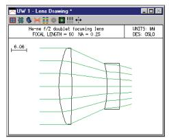
To run a tolerance analysis on a lens, use a copy of the lens, not the original file. OSLO uses the same data structure for optimization and tolerancing, so tolerancing data will overwrite optimization data. After you have opened a saeparate copy of the lens, you should follow the steps below.
