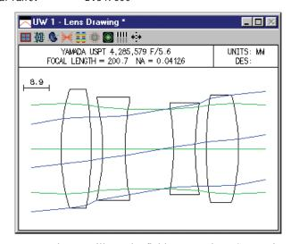
2) For tolerance operands, we will use the field-averaged RMS spot size, computed in three wavelengths. Since this is a rotationally-symmetric lens and we are only perturbing the curvatures, we can use the OSLO error function generator with the default field and pupil sampling options. In the dialog box for the Optimize>>Generate Error Function>>OSLO Spot Size/Wavefront dialog box, accept all the defaults except for the
